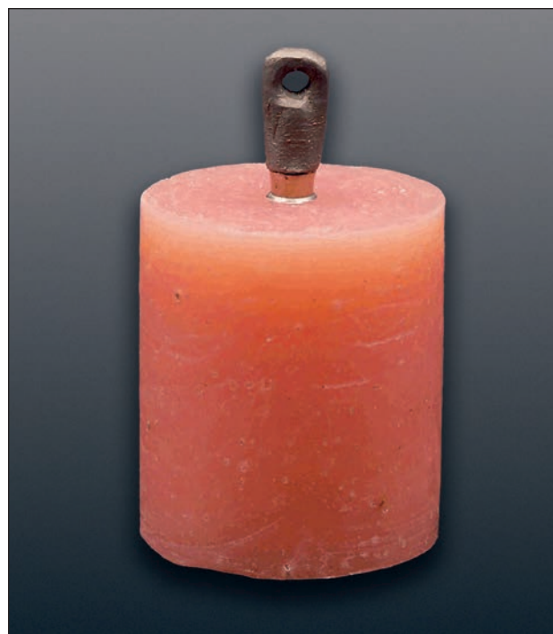
Fig 2 Implant analog with abutment and coping in an acrylic resin block.
