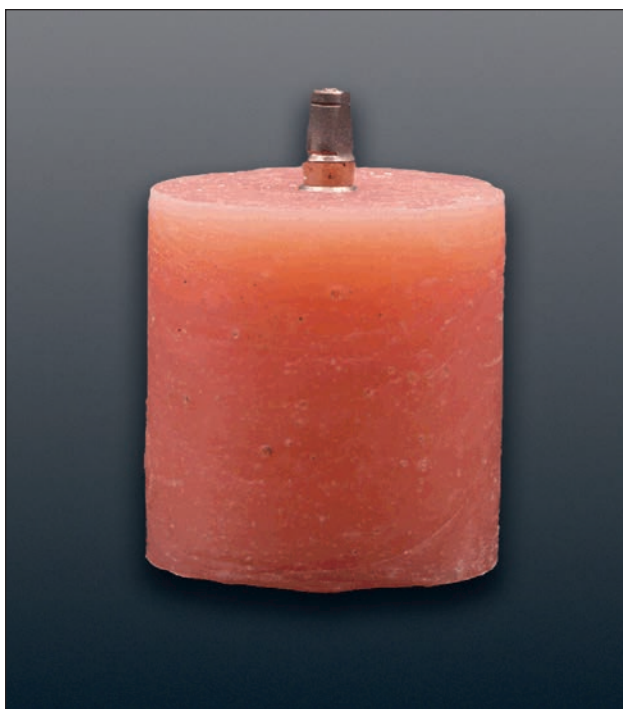
Fig 1 Implant analog with abutment seated in an acrylic resin block.
